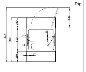
Electric Supply voltage: 322000 (F01H2AW02S) 220-240 V/1N ph/50/60 Hz Electrical power max.: 2.04 kW Water: Water drain outlet size: 3/4" **Key Information:** N° of doors: External dimensions, Width: 770 mm External dimensions, Depth: 1180 mm External dimensions, Height: 1304 mm Net weight: 94.5 kg Shipping height: 1420 mm Shipping width: 910 mm 830 mm Shipping depth: Shipping volume: 1.07 m<sup>3</sup> +85 / +9<u>5</u> °C Set temperature:
